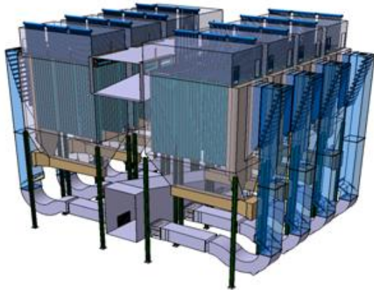
Gas outlet with Louver Dampers
